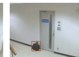
The abandoned bag is detected and indicated by red frame.
